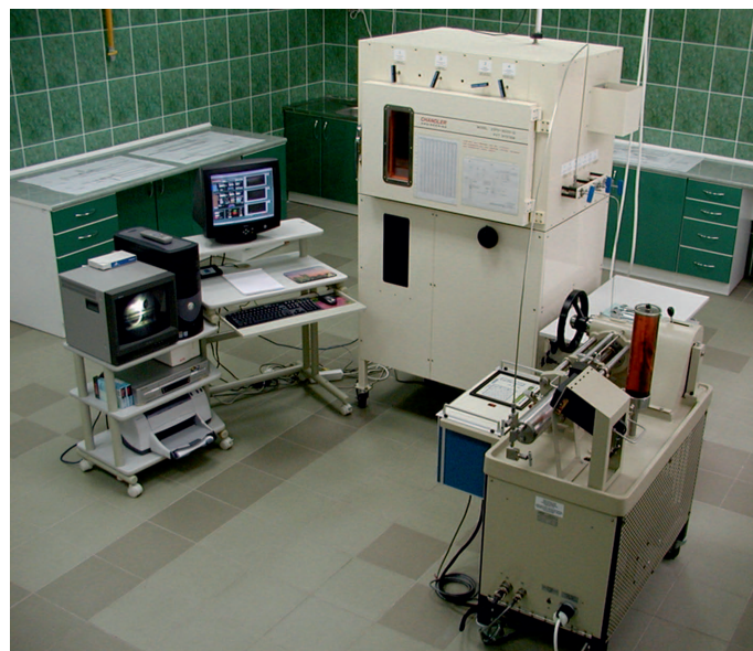
Rys. 2. Aparatura do badań PVT firmy Chandler Engineering – Model 2370-3000-G PVT System (Lubaś et al., 2012)
