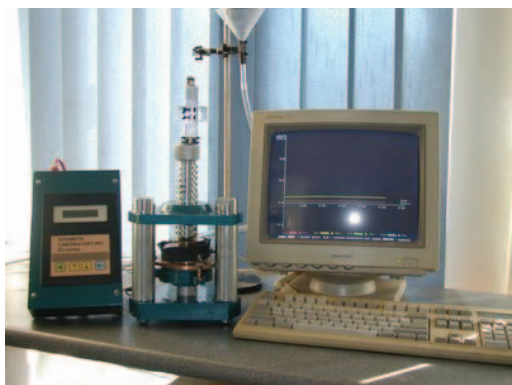
Fig. 4. Apparatus for measuring the swelling pressure of silty rocks and shales (edometer)
